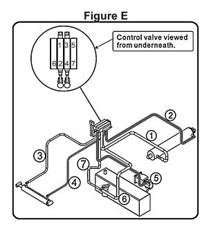
Connect the hoses as marked (Hose 1 to Connection 1, for example) the hoses will only reach the proper connections if attached in the proper orientation - See Figure E. Filling the Hydraulic Fluid
